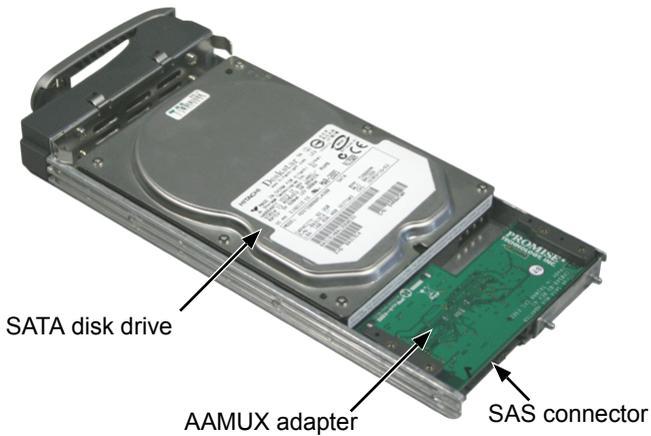
**Figure 10. SAS drive mounted in a drive carrier**
