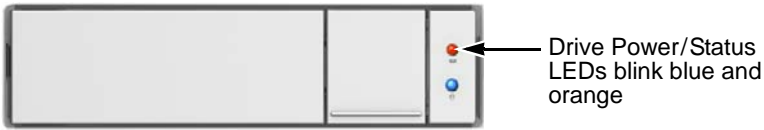
Figure 11. Running the Locate function to identify a disk array
