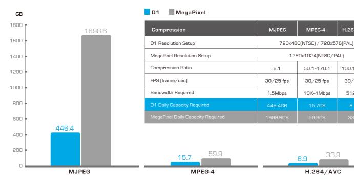
The number of daily capacity required was based on the calculation of 24/7 continuous recording with 30/25 video frames stored in a second to hard disk drives. Any change on resolution, code selection, FPS setup for various record conditions will result in a different storage need.
