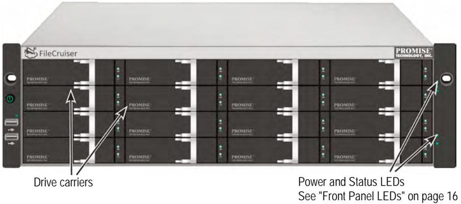
A defective drive may be replaced without interruption of data availability to the host computer. The self-contained hardware-based RAID logical drive provides maximum performance in a compact external enclosure.
