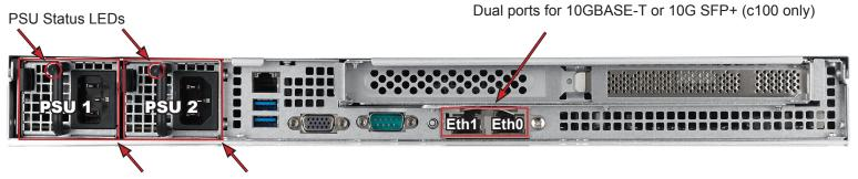
Two Power Supply Units (1+1 Redundant PSU)
