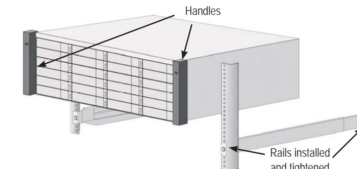
3. Secure the enclosure to the rack.
