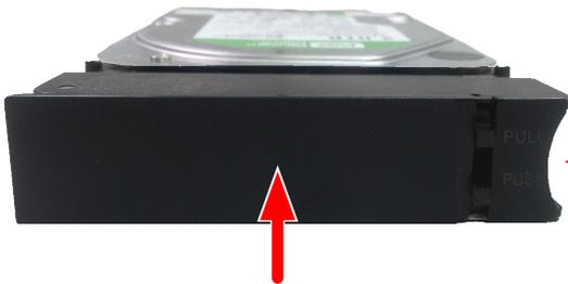
Pull handle to release the latch, then pull straight out gripping the handle. Place your free hand underneath when removing or inserting the carrier containing a hard disk drive, so you do not drop it.
