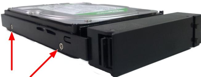
Counter sink screws; two screws on each side.
