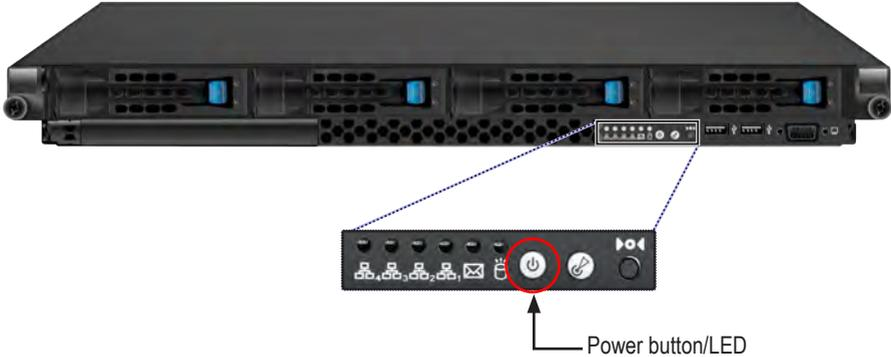
To power on the FileCruiser Server 1U4 simply press the Power button on front of both devices. Power on both units and check the Power LED and other LEDs to monitor the boot up process.
