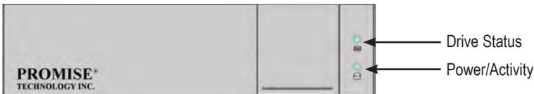
If there is a disk drive in the carrier, the Power/Activity LED displays Blue. If not, the Power/Activity LED remains dark. The Power/Activity LED flashes Blue during drive activity.
