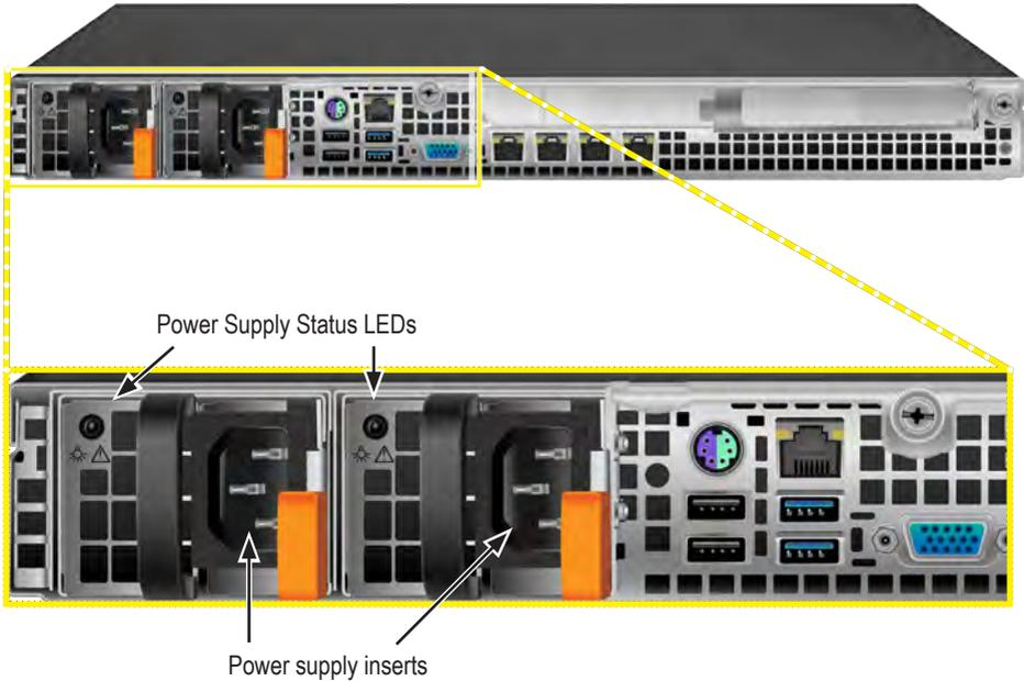
With the power supplies connected, the system can now be powered on. Again, note that if your setup includes a SAN, DAS or cascade with Vess J2600 expansion, always power on the JBOD subsystems first.
