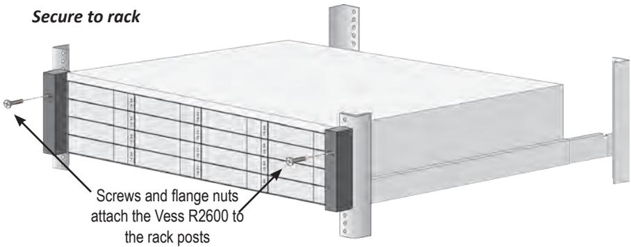
**Subsystem installed in rack**
