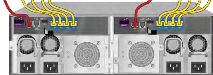
The management network path represented by the red colored cable in the illustration above, is used to configure the Vess R2600iD for operation with the FileCruiser Server 1U4. Once configured, this port is not used for ongoing operations, but it is a good idea to keep the cabling in place for future administration of the Vess R2600iD.
