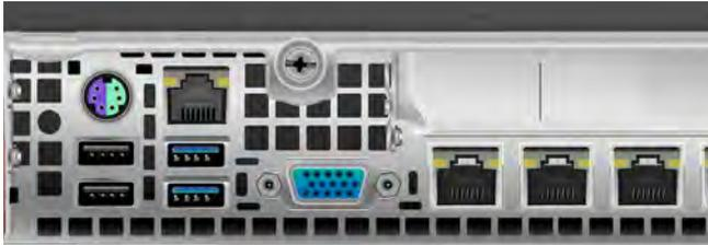
Use any USB port or the PS/2 port to connect a keyboard. Use the VGA port to connect a monitor. Turn on the monitor and the server is ready to be powered on.
