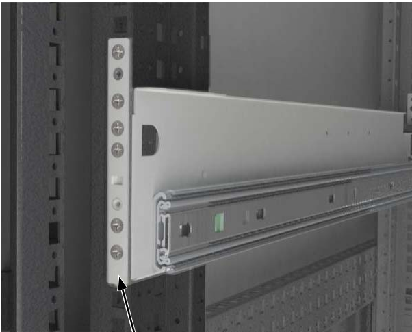
Rack rail attached at the front the rack
