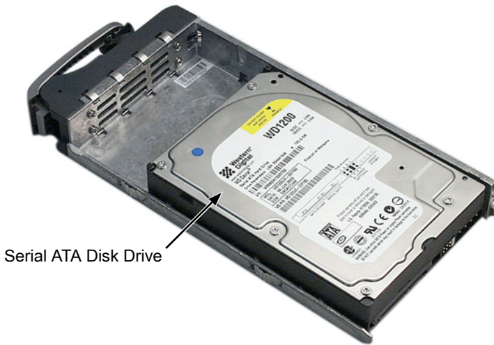
Figure 5. SATA Disk Drives mount at the front of the carrier
