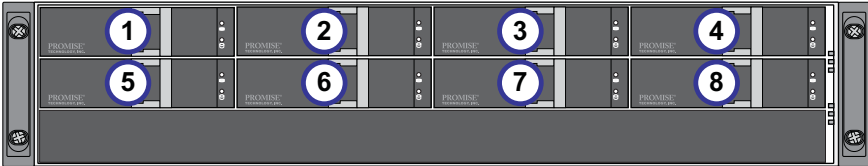
Figure 7. 8-bay VessRAID drive slot numbering
