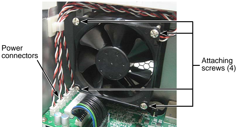
Figure 5. RAID Controller cooling fan
