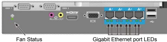
Figure 22: Vess control panel LEDs
