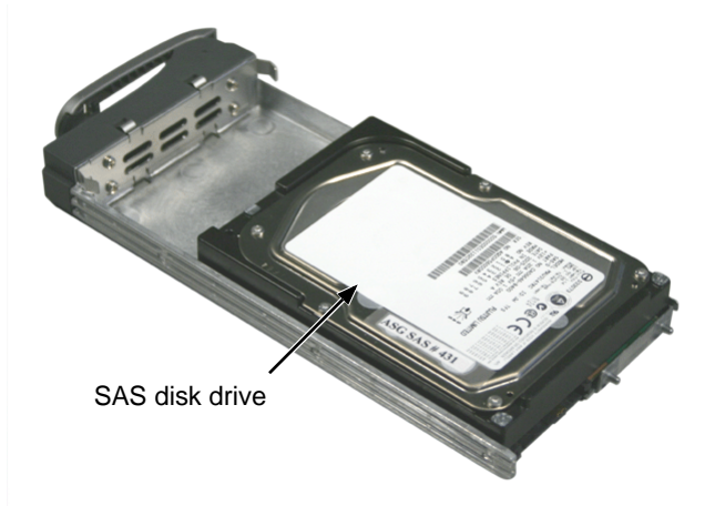
Figure 7. SAS drive mounted in a drive carrier
