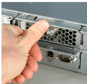
Figure 12. Locking the cooling unit handle (left: E610f/s, right: E310f/s)
