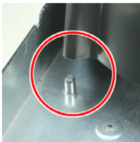
Figure 11. Positioning the blower onto the mounting pins, pointed outward
