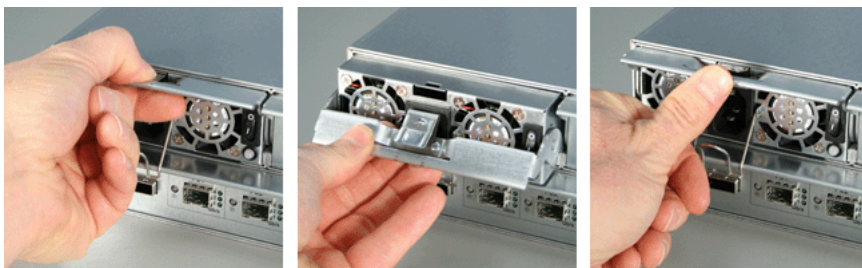
Figure 2. Replacing an E310f/s power supply
