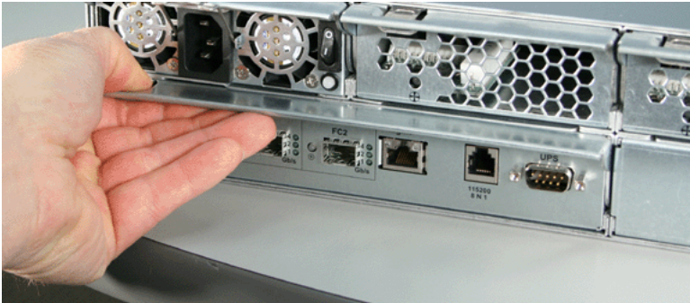
Figure 21. Replacing the controller. The E310f/s is shown. The E610f/s is similar
