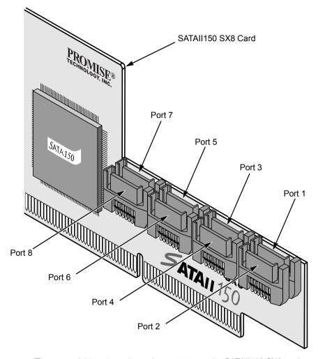
There are eight ports or channel connectors on the SATAII150 SX8 card. The figure above shows how they are numbered.
