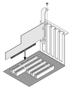
3. Install the SATAII150 SX8 card into the open PCI-X slot (see above). Secure the bracket to the system's frame.
