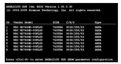
When the SATAII150 SX8 BIOS appears, press Ctrl-F to access the Parameter Configuration.
