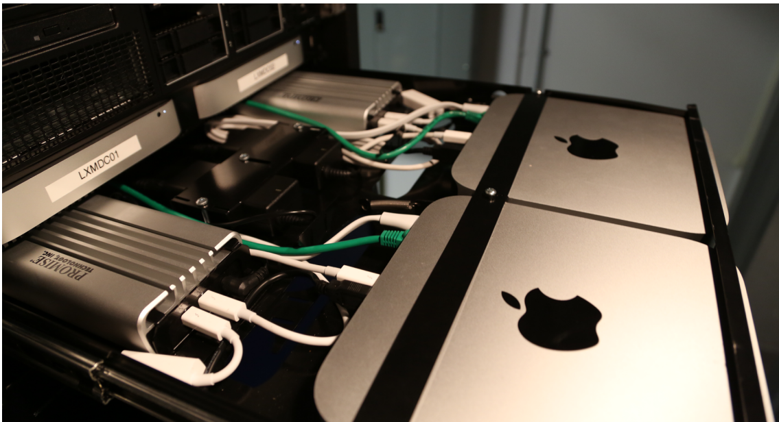
The PROMISE SANLink Thunderbolt to Fibre Channel bridge connect NBC's Mac minis to the VTrak J930s
