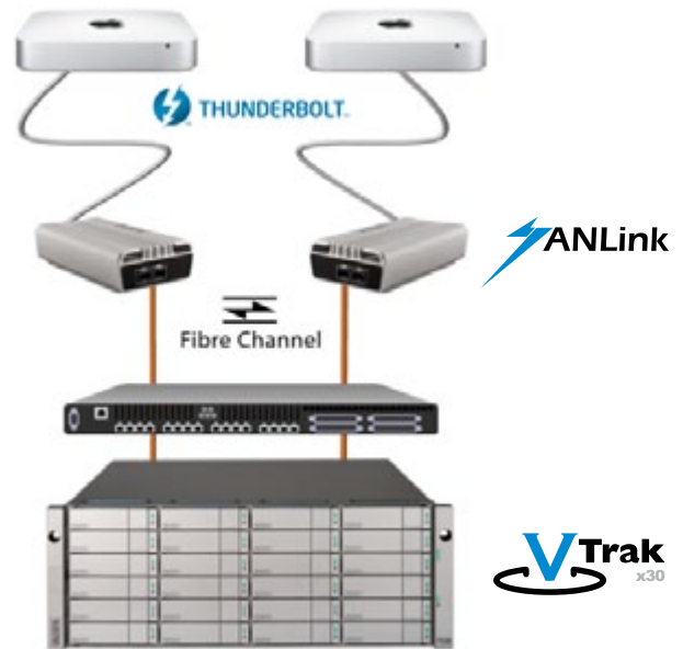
Figure 1. Xsan metadata controller setup with SANLink Thunderbolt to Fibre Channel adapters connected to VTrak x30 Series RAID Storage.
